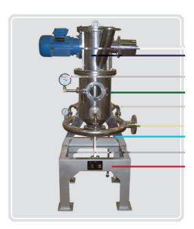
Fine materials in line with size requirements go into cyclone separator and dusting filter through classifying wheels, while coarse materials fall down to crushing chamber to be crushed continuously
